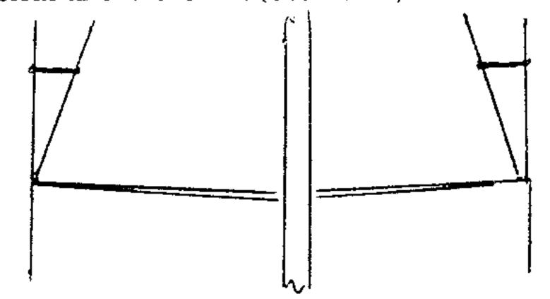
Use more 1/8 inch Dacron cord to create netting between deck and upper lifeline forward of the mast. Instead of making holes in the toe rail, start yhour net by stringing a piece of the 1/8 Dacron or some Kevlar cord, very tightly between the base of the pulpit and the 1st and 2nd stanchions back. Then lace into that as you would the top lifeline and middle lifeline with a series of three clove hitches or modified rolling hitches between uprights. (See Below)
