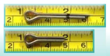
Then simply feed the cord through the pins and tie-on with a square-knot. You can put a lock-stitch through the knot if you are worried about the knot coming out, but shock-cord really locks the knot when you tighten it. The 3/32" pin's eye are a tight fit for the 1/8" cord, so it helps to use a hot knife and cut it on an angle or melt the ends and pinch the end while it's still soft to create a tip to help thread.
